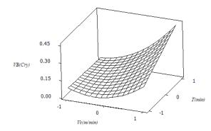
Fig. 1. 3D surface graph for interaction effects of cutting time and cutting speed on the tool life in dry machining
