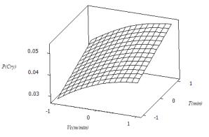
Fig. 5. 3D surface graph for interaction effects of cutting time and cutting speed on power consumption in cryogenic machining
