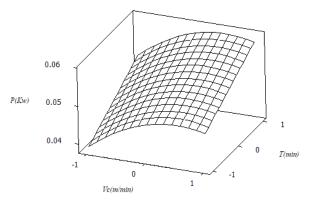
Fig. 4. 3D surface graph for interaction effects of cutting time and cutting speed on power consumption in dry machining
