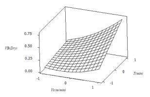
Fig. 2. 3D surface graph for interaction effects of cutting time and cutting speed on tool life in cryogenic machining
