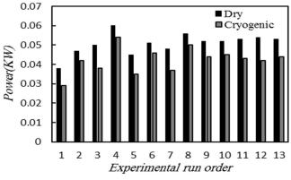
Fig. 6. Comparison of power consumption in cryogenic and dry turning
