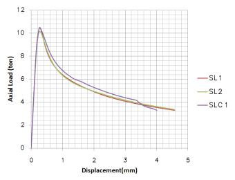
Fig. 7. FEM load-displacement curves
