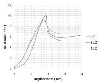
Fig. 5. Experimental load-displacement curves
