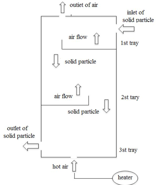
Fig. 2. Schematic view of the new design of three-story dryer
