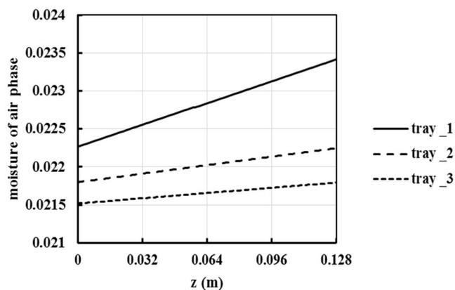
Fig. 4. Change of air moisture in the height of trays
