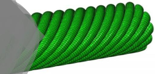
Figure 2. Mesh description of the 1×27 SMA cable.
