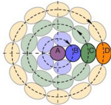
Figure 1. Cross section of 1×27 SMA cable [2].
