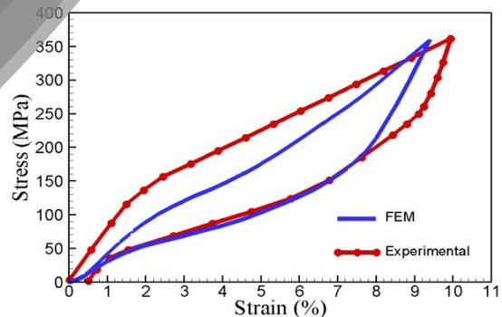
Figure 3. Comparison of normal stress-strain response in present work and experimental data [2].
