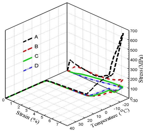
Figure 5. The normal stress-strain-temperature response of 1x27 cables components.
