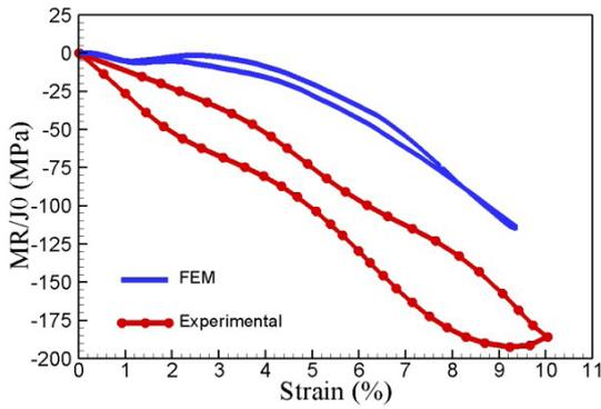
Figure 4. Comparison of shear stress-strain response in present work and experimental data [2].
