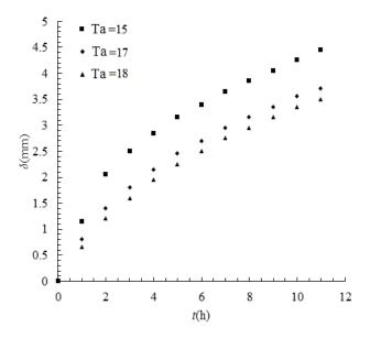
Fig. 5. Frost thickness on top of cylinder at  $T_p$ =-14.6°C,  $\Phi$ =36%, u=0.6 m/s and different surrounding air temperatures
