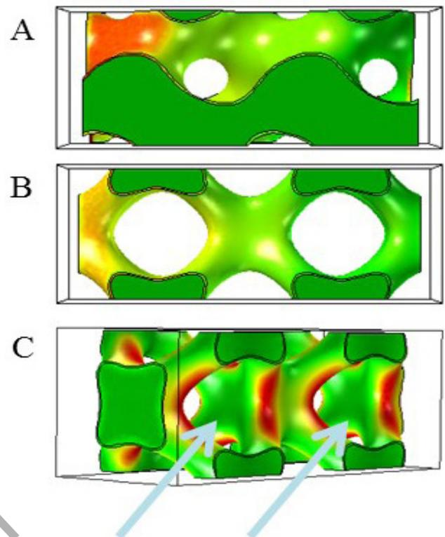
**Figure 2. Von Mises stress distribution in: (A) Scaffold G; (B) Scaffold I; and (C) Dead zone in scaffold I.**
