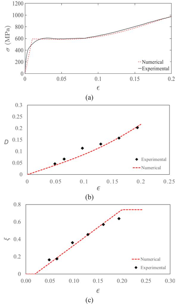
**Fig. 1. Comparison of the numerical and experimental results for plastic behavior of AISI 304 stainless steel at cryogenic temperature**
