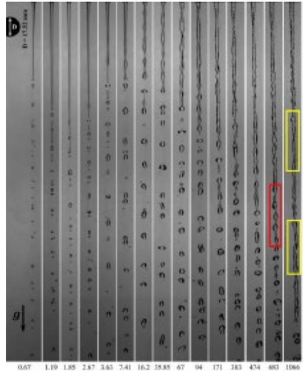
Fig. 2. Elliptical jet visualization for different Weber numbers
