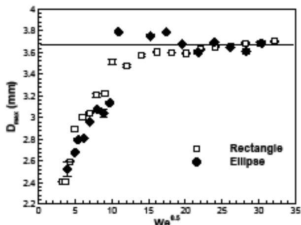
Fig. 5. Variation of axis-switching amplitude with  $We^{0.5}$
