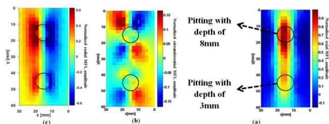
Fig. 2. MFL C-scans for the nearby pits with the spacing of 20 mm: (a) axial signal, (b) tangential signal, and (c) radial signal
