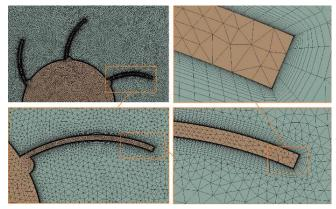
Fig. 2. Fine mesh around the complex geometry
