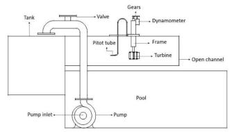
Fig. 1. Schematic side view of the experimental setup In this study, the non-dimensional characteristics of the flows are shown in Table 1:
