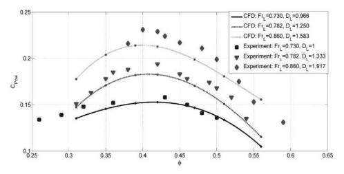
Fig. 4. Power coefficient versus flow coefficient curves-FS cases.
