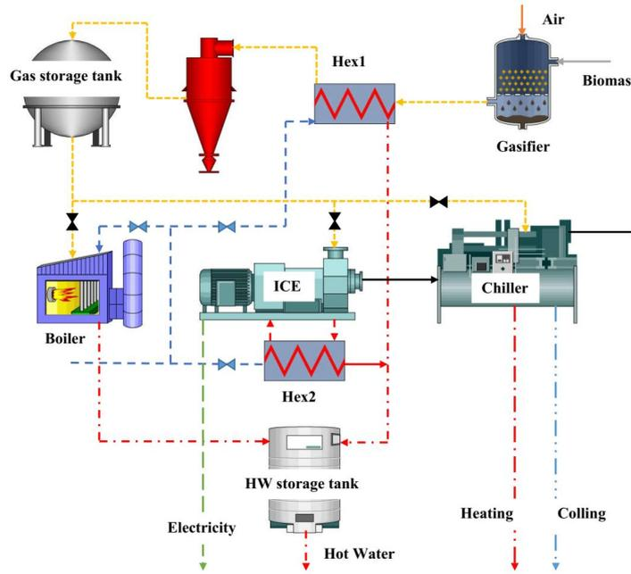
Fig. 1. Cogeneration system connected to biomass gasifier
