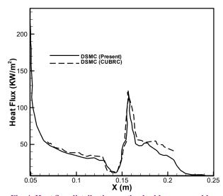
Fig. 4. Heat flux distribution on the double cones problem
