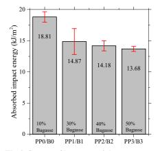
Fig. 3: The influence of bagasse weight percentage on the specimen absorbed impact energy
