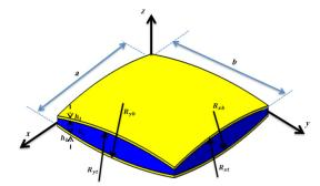
Fig. 1. The geometry of the studied doubly curved sandwich panel The relation of the core thickness can be defined as follows:
