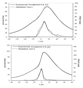
Fig. 1. The validation of in-cylinder pressure and heat release rate for both cases [4].
