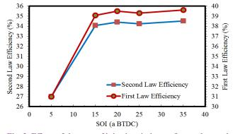
Fig. 3. Effects of the start of injection timing on first and second low Efficiency
