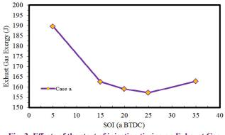
Fig. 2. Effects of the start of injection timing on Exhaust Gas Exergy
