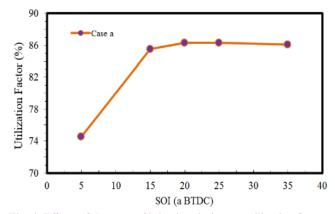
Fig. 4. Effects of the start of injection timing on utilization factor
