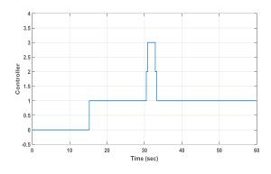
Fig. 2. scheduling controller designed for the nonlinear model of the aircraft  $K_{formal} = 0, K_1 = 1, K_2 = 2, K_3 = 3, K_{safe} = 4$
