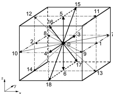
Fig. 2. Discrete velocity vectors for D3Q19.
