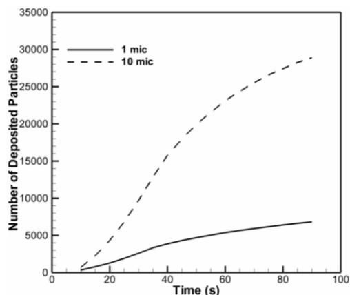
**Fig. 5. Number of deposited particles on the various surfaces for inlet air location on the floor.**
