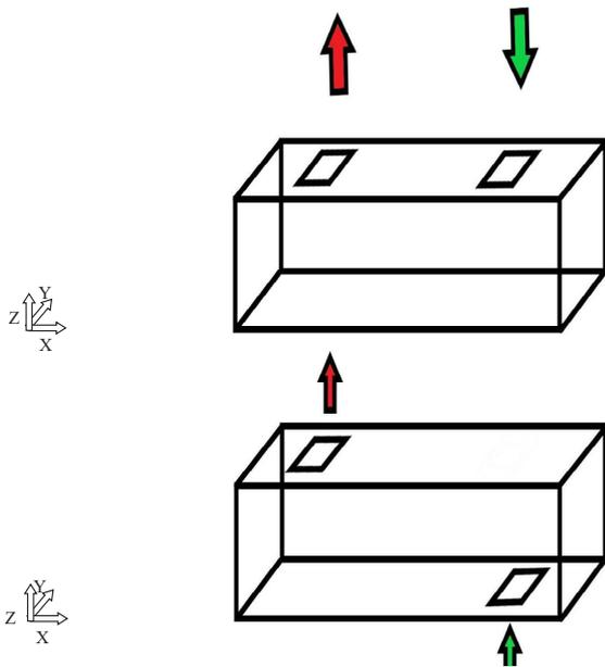
Fig. 1. Geometry of the scaled room studied.
