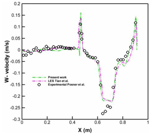
Fig. 3. Vertical velocity along the horizontal line at mid-partition height from the left wall to the right wall
