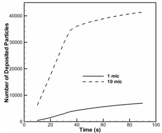
Fig. 4. Number of deposited particles on the various surfaces for the inlet air register on the ceiling.
