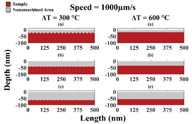
Fig. 2. Comparison of nanomachined final surface with base excitation at 300 °C and 600 °C at tip radius (a) 5nm, (b) 20nm, (c) 40nm and at speed of 600
