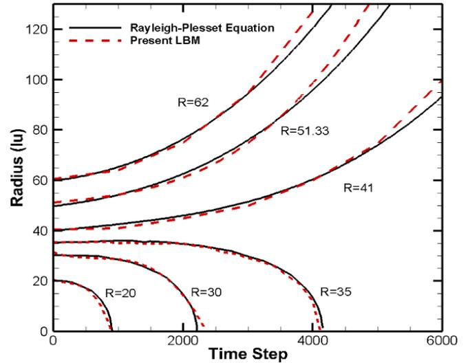
**Fig. 1. Comparison of the results obtained by C-S EOS and revised Rayleigh-Plesset equation for the gradual change in the size of non-homogeneous cavitation bubbles at  $\Delta P = -0.0595$  and  $R_c = 37.2$**
