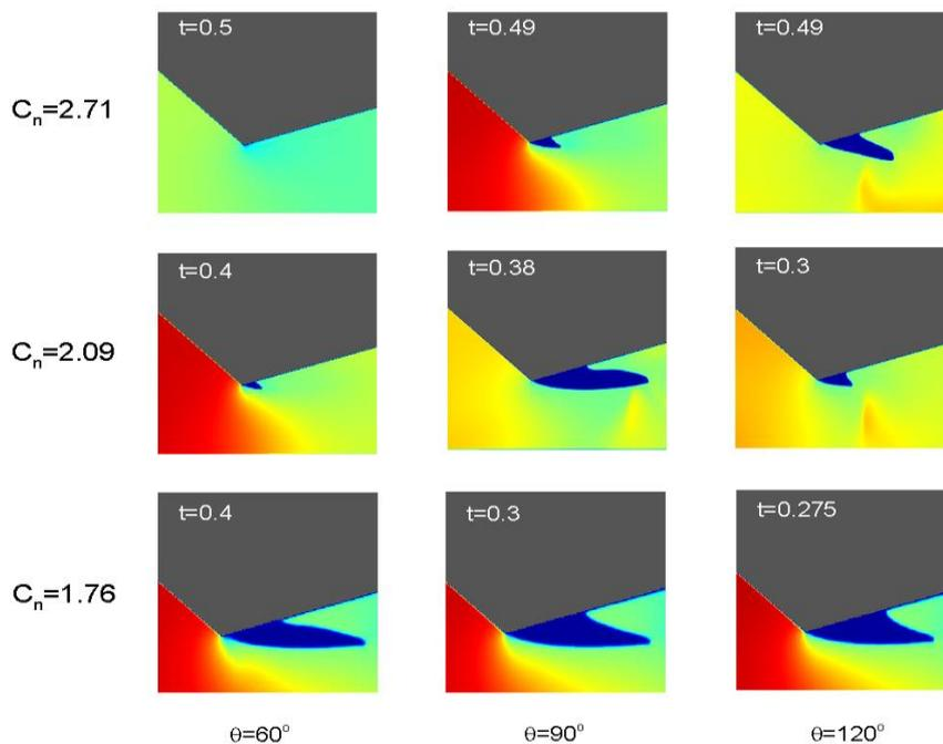
**Fig. 2. Comparison of cavitation zone formed in convergent-divergent nozzle throat, obtained from present numerical solution with SC equation of state in cavitation numbers and different contact angles**
