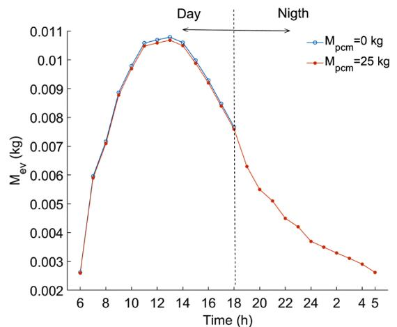
**Fig. 5. Evaporation mass of the moisture in greenhouse dryer affected by the presence and lack of PCM**
