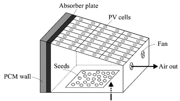
**Fig. 1. Schematic diagram of the investigated greenhouse dryer in the present research**
