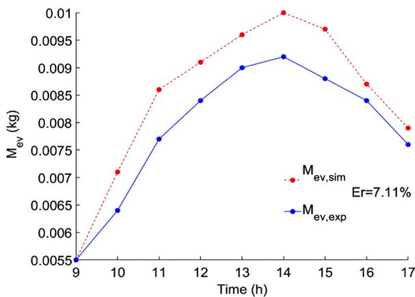
**Fig. 3. Experimental and simulated values of evaporation mass against time of testing**
