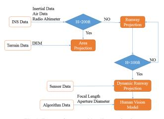
Fig. 1. Frame of proposed landing navigation
