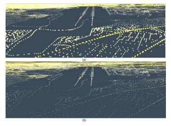
Fig. 2. Simulation of flight area: (a) with depth perception cue; (b) without depth of field
