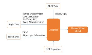
Fig. 3. Block diagram of the depth perception cue implement
