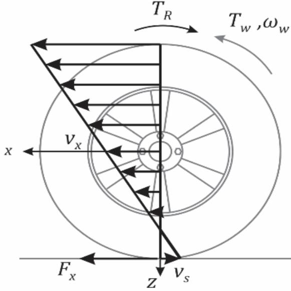
Fig. 1. Free body diagram of the wheel
