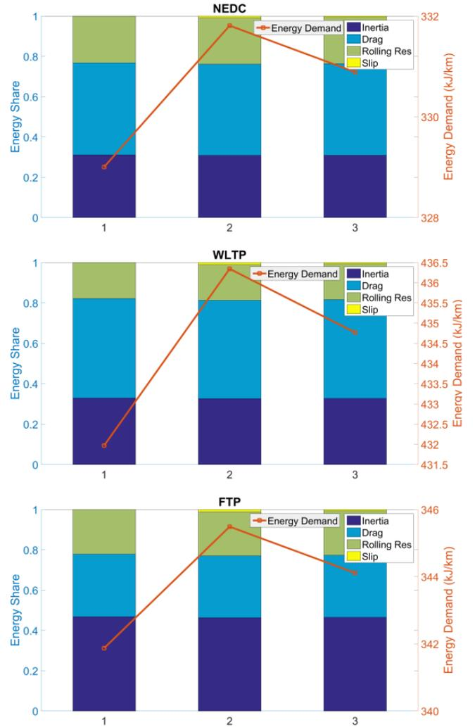
Fig. 2. Energy demand and share of each resistance for compact B-class sedan, 1: neglecting the slip loss, 2: considering the slip loss using physical tire model, and 3: considering the slip loss using verified tire model
