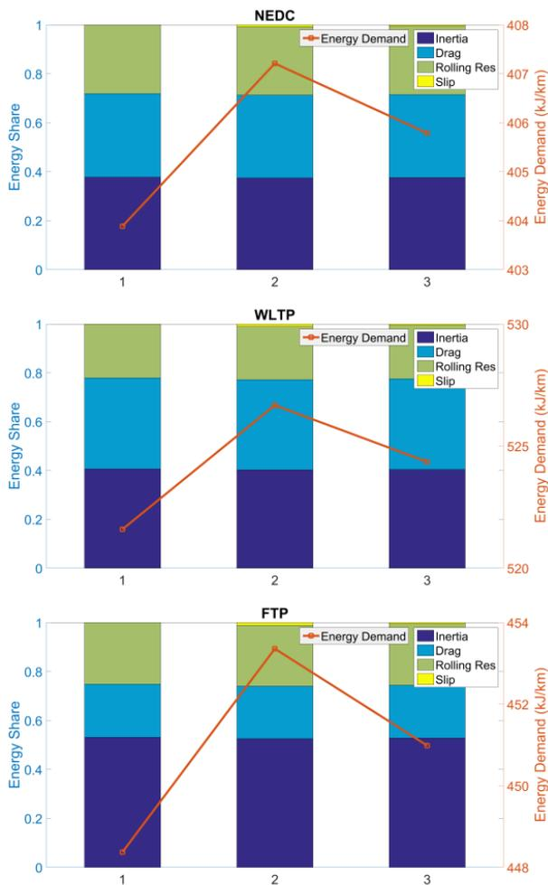
**Fig. 3. Energy demand and share of each resistance for mid-size D-class sedan, 1: neglecting the slip loss, 2: considering the slip loss using physical tire model, and 3: considering the slip loss using verified tire model**
