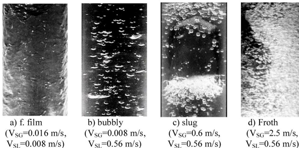
Fig. 1. Processed photos of different flow patterns
