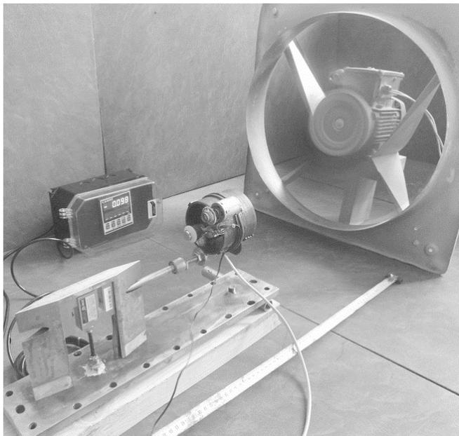
Fig. 1. Experimental setup for test of the wind turbine in the wind flow
