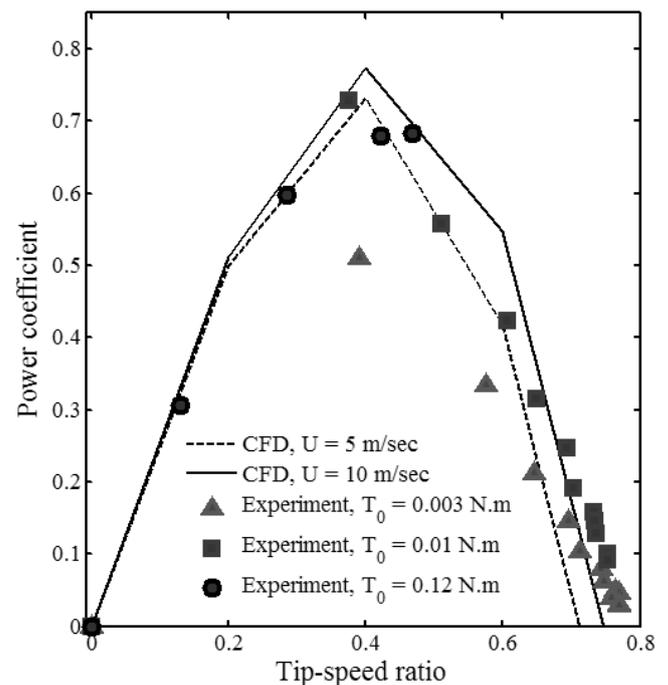
Fig. 2. Experimental and numerical data for power-coefficient of wind turbine against tip-speed ratio
