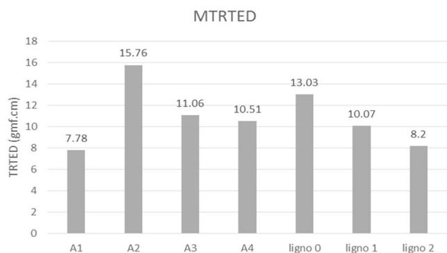
Fig. 4. Maximum Torsional Resistance at Targeted Embedment Depth (MTRTED) of mud cake in the experiments
