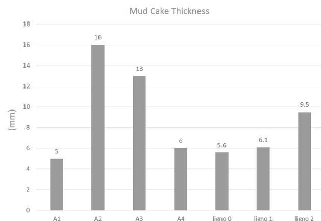
**Fig. 3. Measured thickness of mud cakes**
