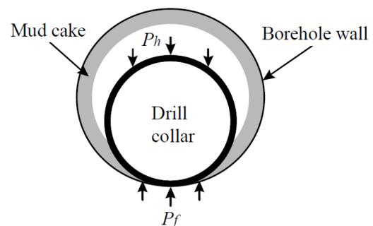
**Fig. 1. Differential sticking.  $P_h$  is the hydrostatic pressure and  $P_f$  is the formation Pressure [2].**
