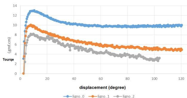
Fig. 5. Torsional Resistance at Targeted Embedment Depth of Lignosulfonate mud cakes
