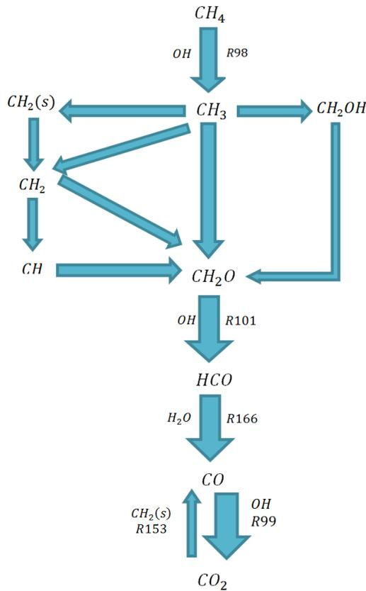
Fig. 1. Reaction pathway diagram for combustion of methane in a well-stirred reactor
