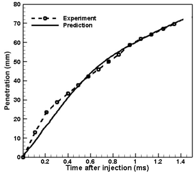
Figure 3. Comparison of experimental [10] and predicted spray tip penetration for  $P=25$  bar and  $T=673$  K
