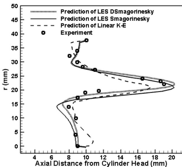
Figure 2. Comparison of axial mean velocity in 36 degrees ATDC at the distance 10 mm from the cylinder head with different turbulence models
