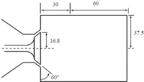
Figure 1. Schematic of Internal Combustion Engine (ICE) geometry
