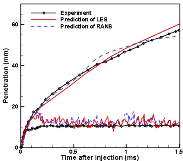
Figure 5. Comparison of reacting liquid spray and fuel vapor penetration length using different turbulence method with experimental data [11]
