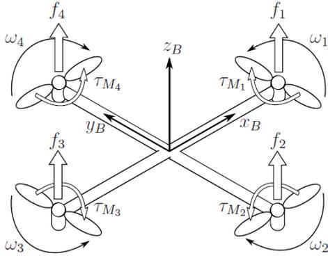
Fig. 1. Schematic view of a quadrotor system
