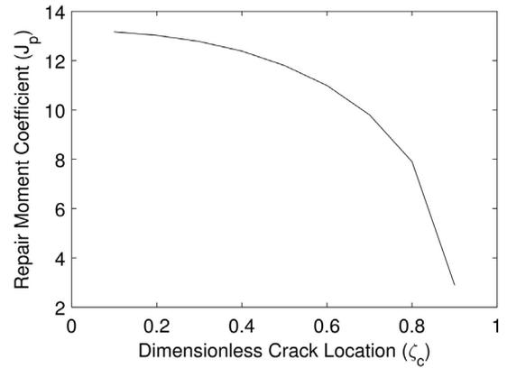
Fig. 3. Effect of the crack location on the repair moment coefficient
