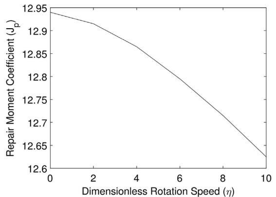
5- Fig. 4. Effect of the rotation speed on the repair moment coefficient
