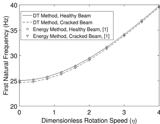
Fig. 2. Effect of the rotation speed on the fundamental natural frequency of a healthy and cracked beam
