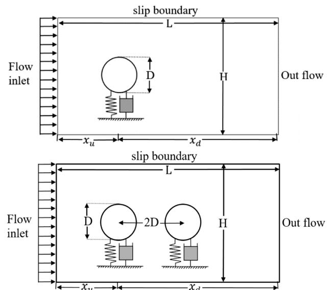
Fig. 1. The computational domain used in this study
