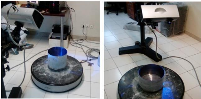
**Fig. 2. 3D scanner camera**
