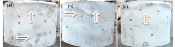
**Fig. 4. Buckling deformation of the shell specimens (a) SL1; (b) SL2; (c) SLC1**
