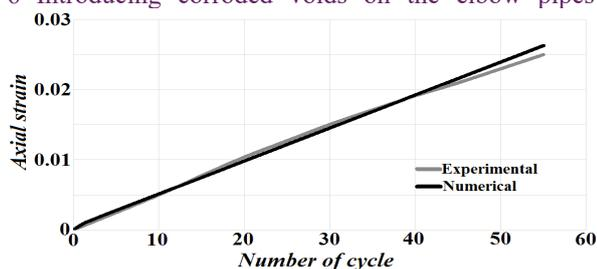
Fig. 1. Comparison of the numerical and experimental results for axial ratcheting on the intrados place.
