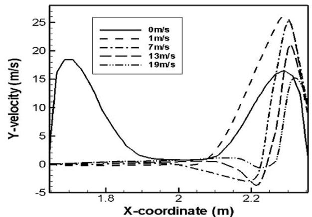
Fig. 4. Variation of vertical velocity over the subway train roof for different train speeds
