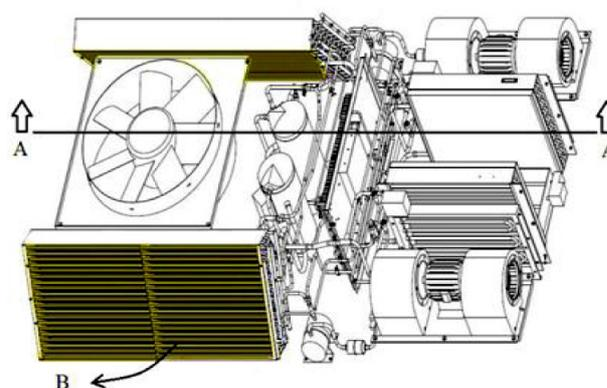
Fig. 1. View of air conditioning system in subway train
