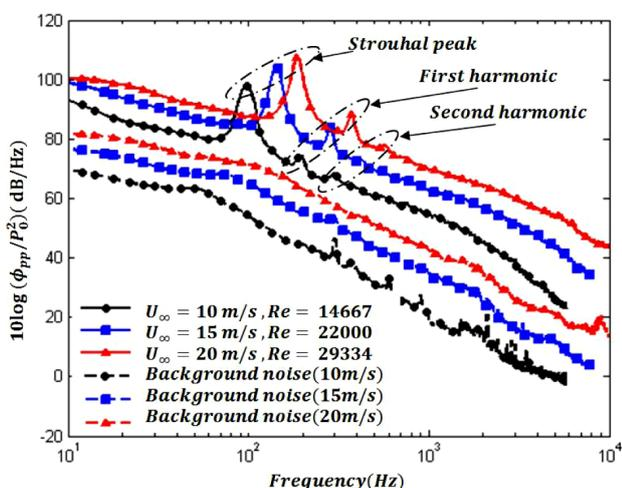
Fig. 2. Surface pressure spectra at  $z/D=0$  and along with wind tunnel background noise
