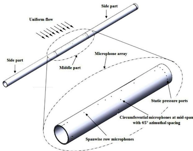
Fig. 1. Cylindrical model including array of microphones on the middle part
