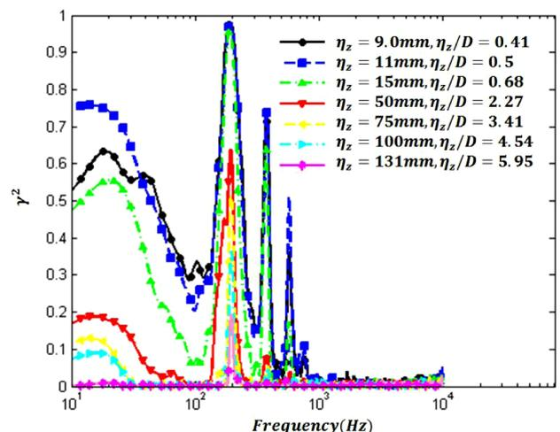
Fig. 3. Lateral coherence variations for various spanwise distances at 20 m/s
