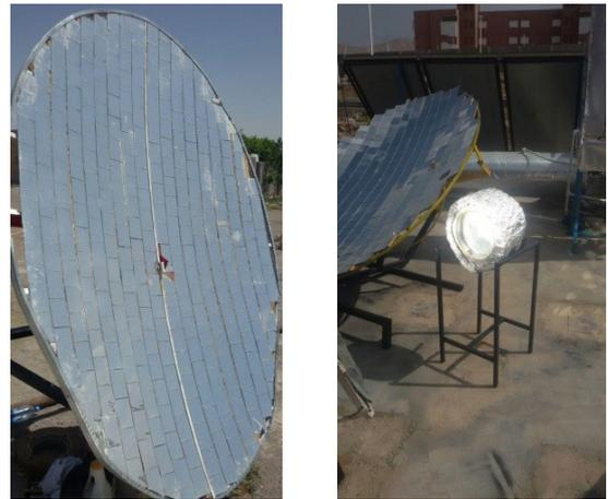
Fig. 4. A view of the manufactured Scheffler concentrator with its receiver
