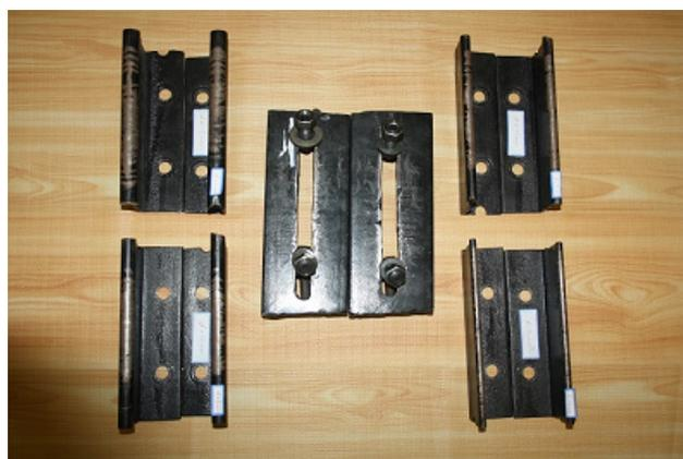
Fig. 1. The fixture of adjustable indenters.
