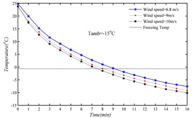
Fig. 3. Temperature distribution in finger-tip under the Wilson et al. [5] conditions at  $-15\text{ }^{\circ}\text{C}$  ambient temperature and different wind speeds
