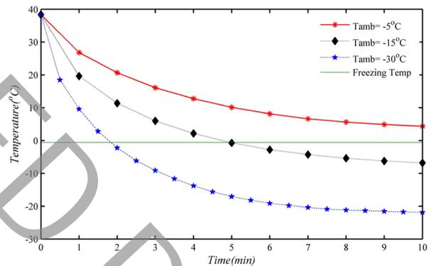
Fig. 4. Temperature distribution in finger-tip at 3m/s wind speed and different ambient temperatures
