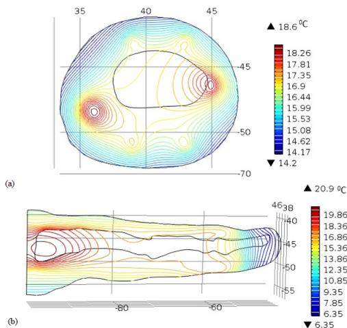
Fig. 2. Isothermal contours at 50 min, in  $-50\text{ }^{\circ}\text{C}$  and 1m/s wind speed a) Axial section at 28.5 mm apart from finger base and b) Sagittal section at the middle
