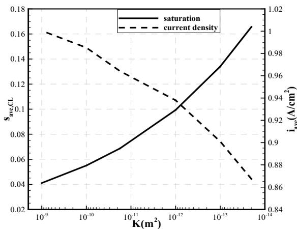
Fig. 2. The effect of GDL permeability on the average liquid water saturation at the CL and the average current density ( $V_{cell}=0.16$  V).
