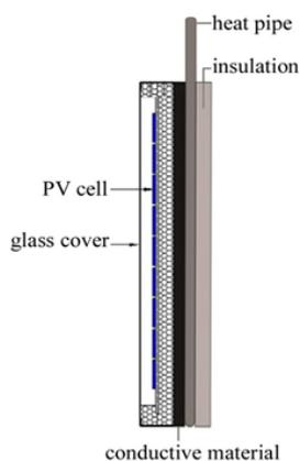
Fig. 1. A schematic diagram of PV module, heat pipes, and an insulating surface
