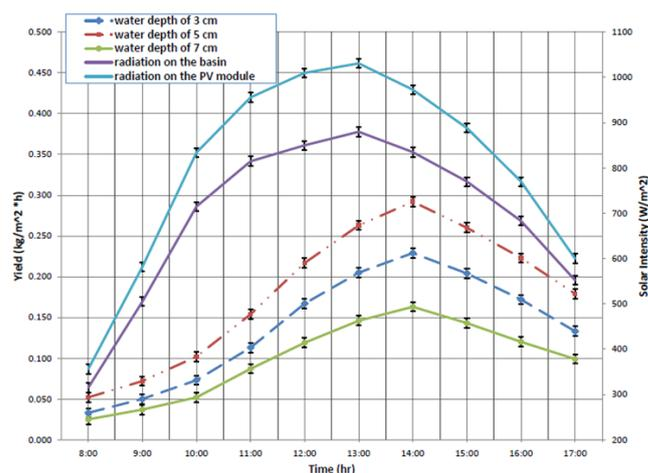
Fig. 3. Solar intensity and the amount of produced freshwater for various water depths in the basin (depths of 3, 5 and 7 cm)
