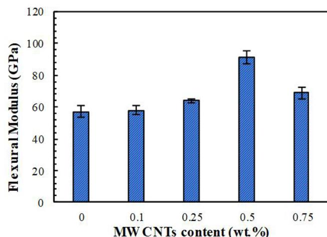
Figure 2. The flexural modulus of basalt fibers/ epoxy/ aluminum 2024 laminates as a function of MWCNTs content.
