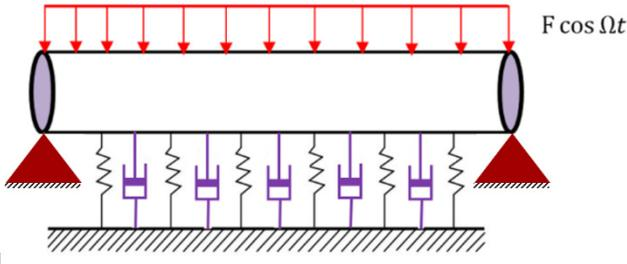
**Fig. 1. Schematic of carbon nanotube under viscoelastic foundation**
