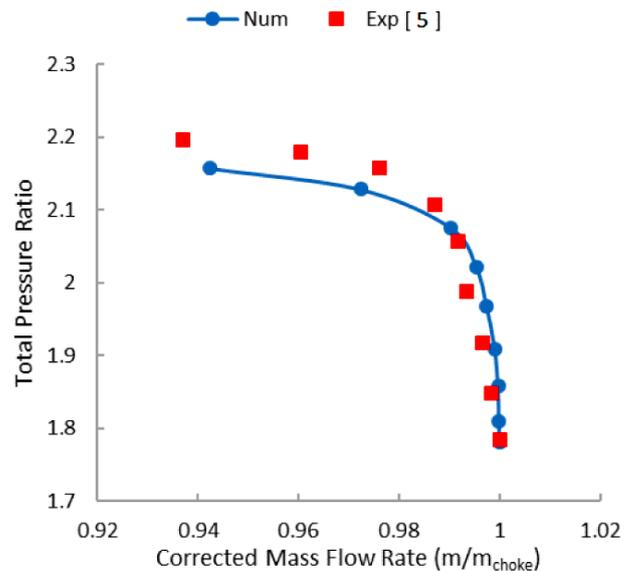
Fig. 3. Compressor performance total pressure ratio curve
