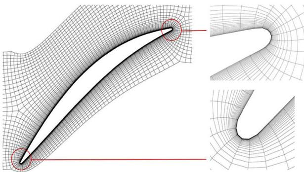
Fig. 2. Rotor blade meshing near hub region
