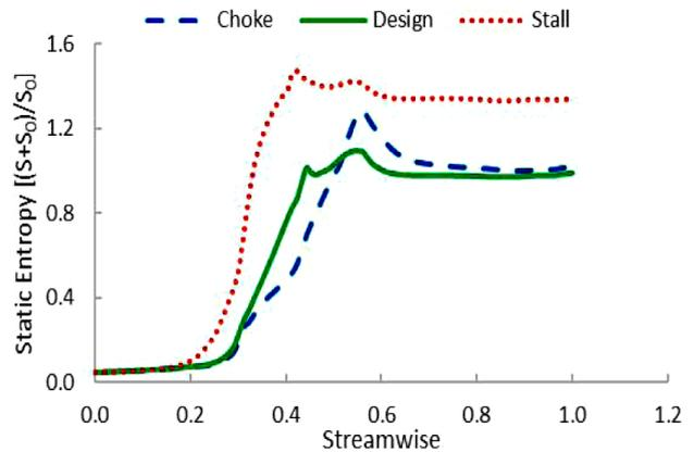
**Fig. 5. Static entropy changes along the flow direction in different performance conditions**
