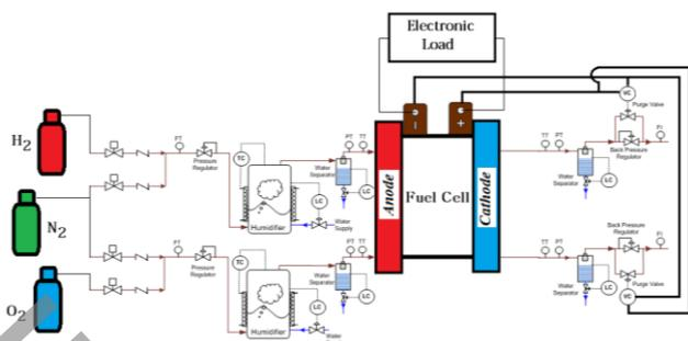
Fig. 1. Process flow diagram of applied test bench
