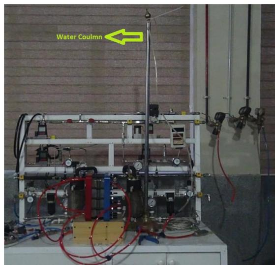
Fig. 2. Hydrating of stack before activation process
