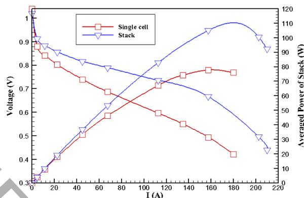
Fig. 3. Comparison of voltage and power of stack and single cell
