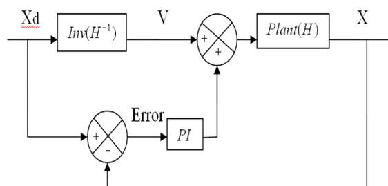
Figure1-Structure of closed loop controller
