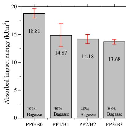
Fig. 3: The influence of bagasse weight percentage on the specimen absorbed impact energy
