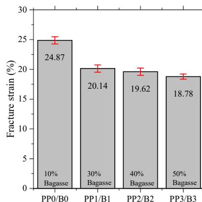
Fig. 2: The influence of bagasse weight percentage on the specimen fracture strain
