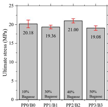
Fig 1: The influence of bagasse weight percentage on the specimen ultimate stress
