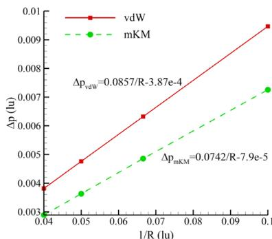
Fig. 1. Laplace test to calculate the surface tension of the droplet.
