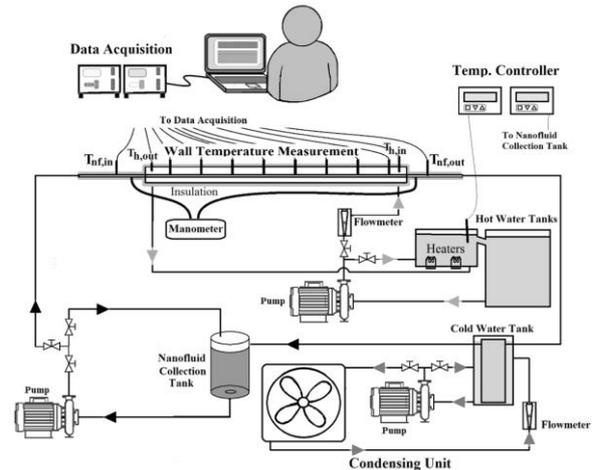
Fig. 1. Schematic diagram of the experimental apparatus.
