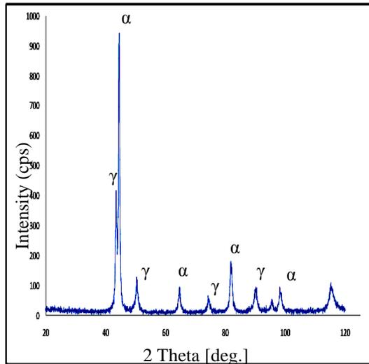
Fig.2 X-ray diffraction pattern of SDSS and WM.
