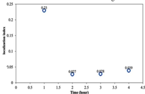
Fig. 3: Localisation index (LI) values of the HSLA base metal/ WM pair calculated for each hour of the ZRA test at ambient temperature.
