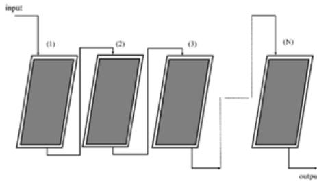
Figure 3. The series connection of collectors
