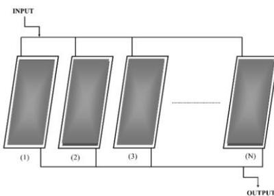
Figure 4. The parallel connection of collectors
