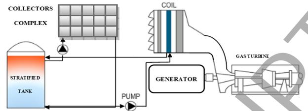
**Figure 1. Schematic diagram of proposed cooling system for compressor's suction air cooling**
