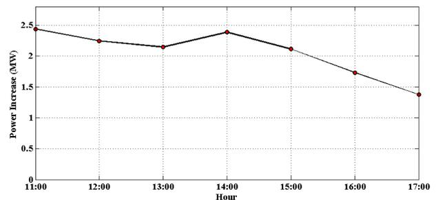
Figure 7. Increased power generation by pre-cooling of the intake air to the compressor with the help of a night radiative cooling system, tank capacity  $1000 \text{ m}^3$
