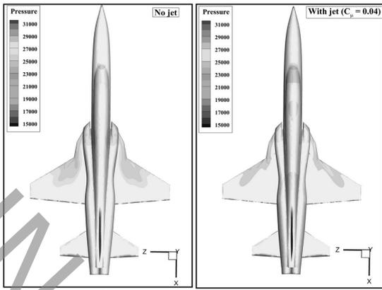
Fig. 3. Static pressure contours on the upper surface of the wing at  $\alpha=16^\circ$
