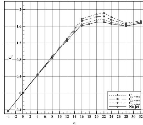
**Fig. 2. The effect of blowing on the lift coefficient versus angle of attack for the bare wing at Mach No=0.4**
